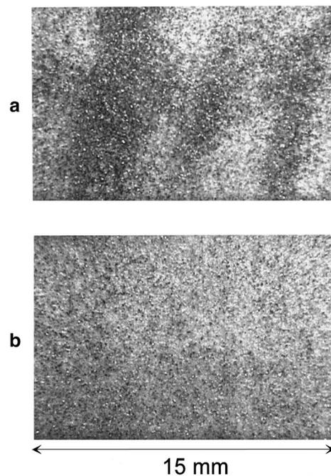
FIG. 4. Illustration of efficient mixing properties of the ascending roll after five rotations of a mixture of different sizes and dark (large) and white (small) particles. Snapshot (a) was taken at the beginning and (b) at the end of the process. A careful analysis of the final product shows that the mixing is practically perfect.
