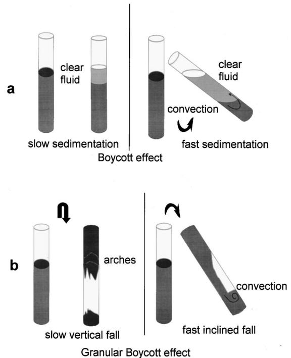
FIG. 1. Sketch showing the analogy between the Boycott effect (a) in sedimentation and the granular Boycott effect (b). In both cases the process is roughly five times faster when the tube is inclined rather than vertical. Convective rolls are present in both cases.
