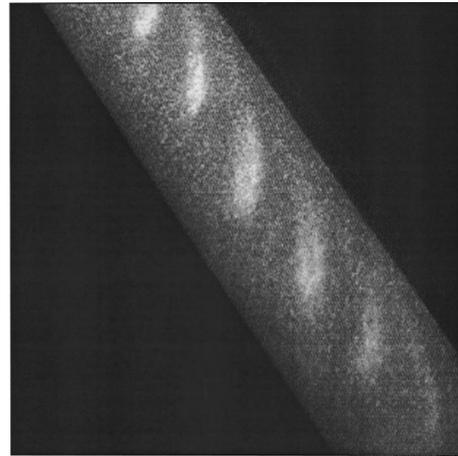
FIG. 3. A luminescent trail left in an inclined tube after a Boycott effect experiment. At the beginning of the experiment, the luminescent powder lies on top of the granular material. This long-time-exposure image was taken after a single rotation of the cylinder. Illumination in the UV shows white zones indicating a high concentration of luminescent powder. Tracking the powder in this way, we find that it is progressively mixed into the granular material.
